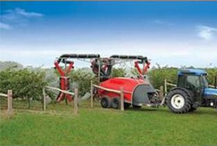
Pumps for orchard airblast spraying for high pressure or low volume treatments
